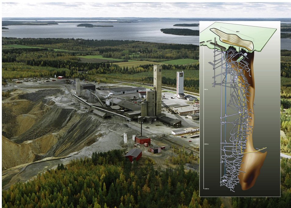
FIGURE 7.6 Aerial and axonometric view of the Pyhäsalmi mine and location map.
